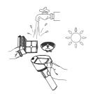
Grasp recessed area on each side of the HEPA and pull upward. Rinse under running water and must be completely dry before recombining with the lid of the DWT.
